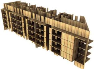
Figure 5: Perspective rendering view of the timber crosslaminated structure of the six storey building
