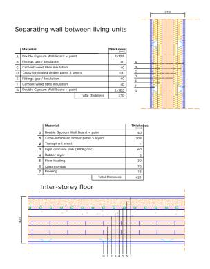
**Figure 4**: Detail of the separating wall between living units and of the inter-storey floor.
